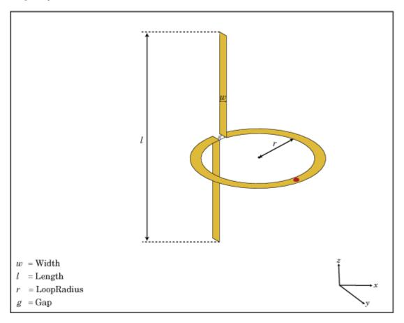
The width of the dipole is related to the circular cross-section by the equation
