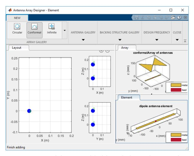
You can view each element separately by clicking on the element in the **Layout** window.
