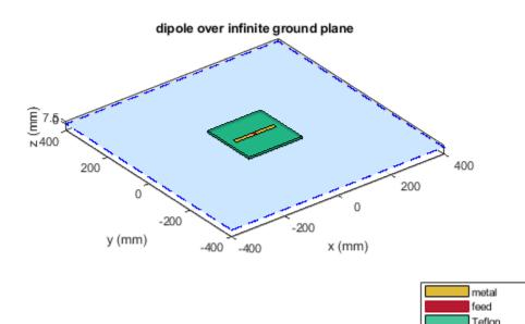
Calculate the radiation pattern of the antenna at 70 MHz. pattern(rf,70e6)
