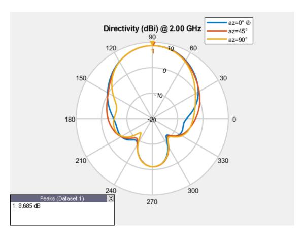
Write the elevation pattern of the helix antenna in an MSI Planet Antenna file.
