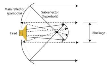
Focus of the main reflector and the near focus of the subreflector in the region between the two dishes. Gregorian antenna forms a shorter focal length for the main dish.
