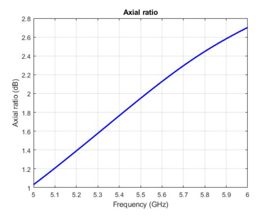
You can see from the axial ratio plot that the antenna supports circular polarization over the entire frequency range.
