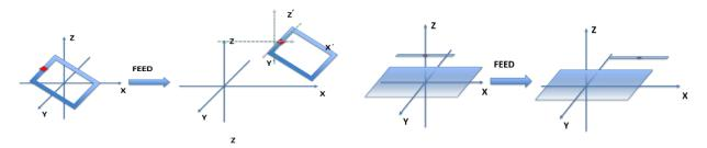
Choosing origin as the position reference moves the antenna element so that new antenna origin is at the specified coordinates. The loop rectangle antenna and reflector-backed antenna show the new position with respect to origin:
