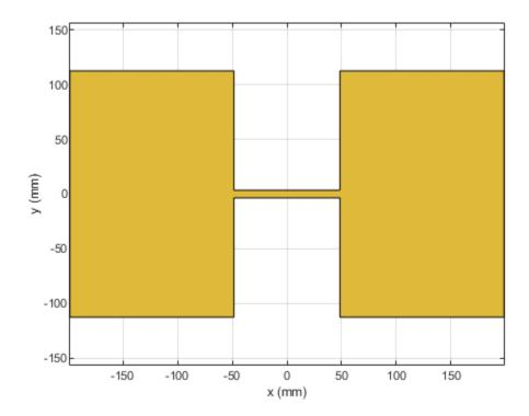
Assign the radiator shape to pcbStack and make the changes to the board shape and feed diameter properties.
