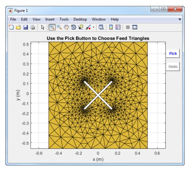
Click **Pick** to display the cross hairs. For an array with two feeds, select two pairs (four points) in the mesh. To specify a feed-region for the, zoom in and select two points each, one inside each triangle on either side of the air gap. Select the points using the cross hairs.
