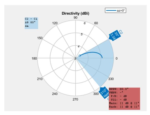
Compare the beamwidth plot and the polar pattern plot. You will see that Antenna Metrics does not represent the beamwidth correctly.
