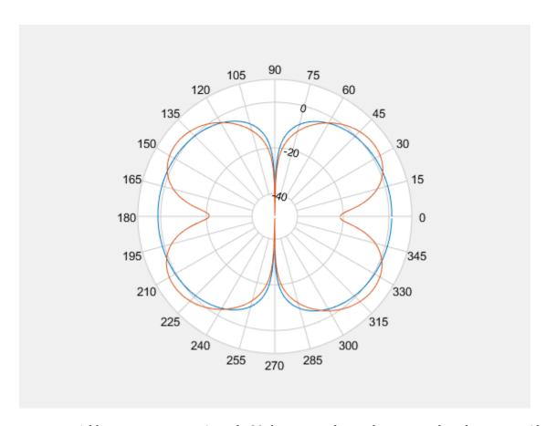
Add a cursor at approximately 30 degrees to the top-hat monopole polar pattern (data set 1) and at approximately 150 degrees to the dipole polar pattern (data set 2).
