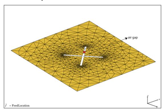
createFeed(antenna) plots a custom antenna mesh in a figure window. From the figure window, you can specify a feed location for the mesh and create a custom antenna.
