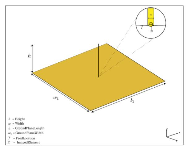
When you load an antenna using a lumped resistor, capacitor, or inductor, the electrical properties of the antennas changes. These lumped elements are typically added to the antenna feed. You can use lumped elements to increase the bandwidth of the antenna without increasing the size of the antenna.
