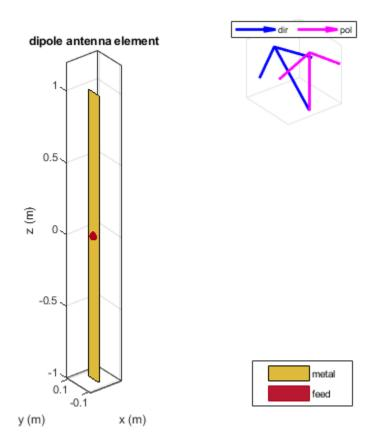
If you use the above option, any analysis of this antenna will error out as the polarization and direction vector are not orthogonal to each other.
