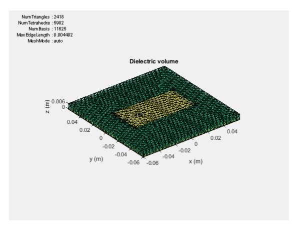
Mesh only the dielectric surface of the antenna.
