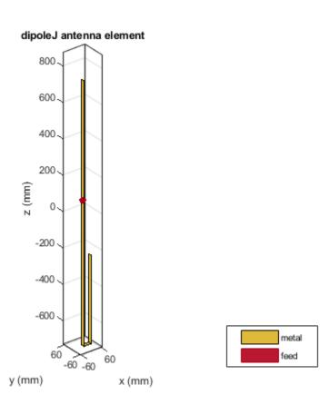
Calculate the impedance of the antenna over a frequency span 140MHz - 150MHz. impedance(dj,linspace(140e6,150e6,51));
