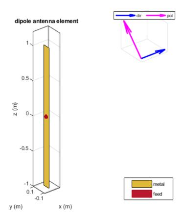
Calculate the current distribution of the antenna. current(p,75e6);
