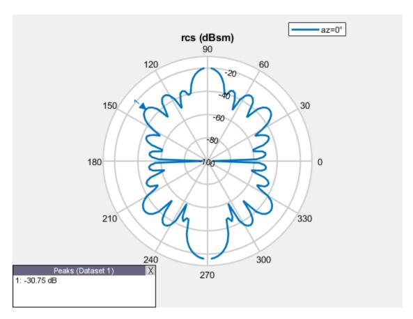
Plot the RCS in the azimuth plane.
