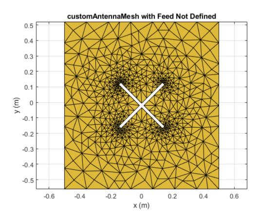
Create the feed for the custom antenna across the points (0.07,0.01) and (0.05,0.05) meters respectively.
