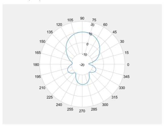
Create a dipole antenna and calculate the directivity at 270 MHz.
