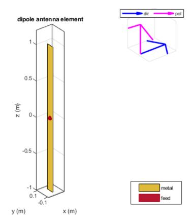
The blue arrow shows the direction of propagation of the plane wave. By default, the direction is along the x-axis. The pink arrow shows polarization of the plane wave. By default, the polarization is perpendicular to the direction of propagation i.e. along the z-axis.
