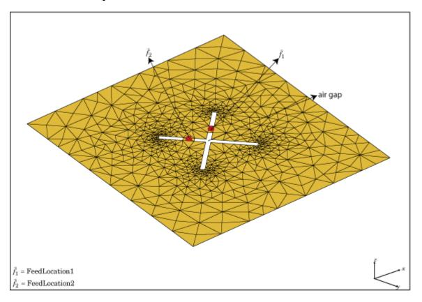
createFeed(array) plots a custom array mesh in a figure window. From the figure window, you can specify feed locations by clicking on the mesh and create a custom array. To specify a region for the feed point, select two pairs of points, inside triangles on either side of the air gap.
