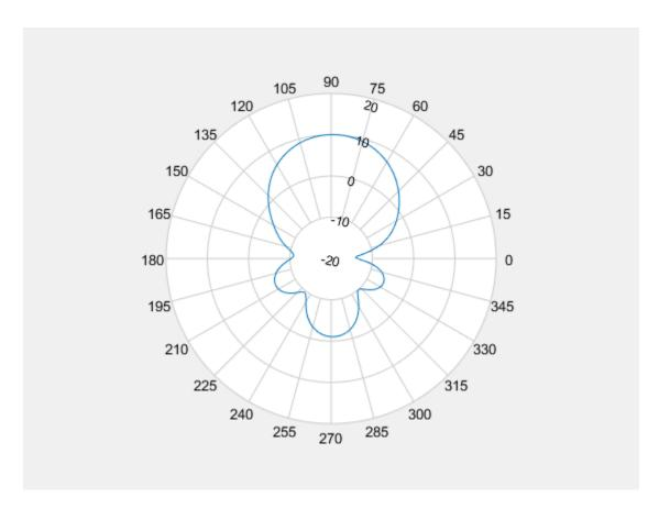
Create a dipole antenna and calculate its directivity at 270 MHz.
