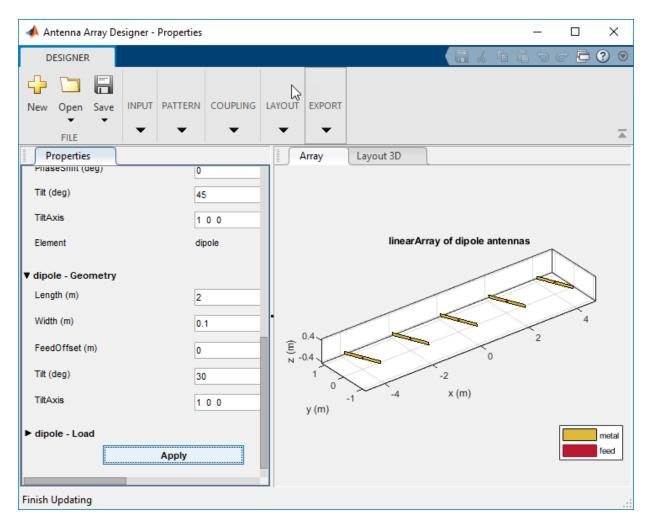
On the **Input** pane, change the **Center Frequency** of the array to 60 MHz. Click **3D Pattern** in the **Pattern** pane to plot the radiation pattern. Observe the maximum directivity of the array.
