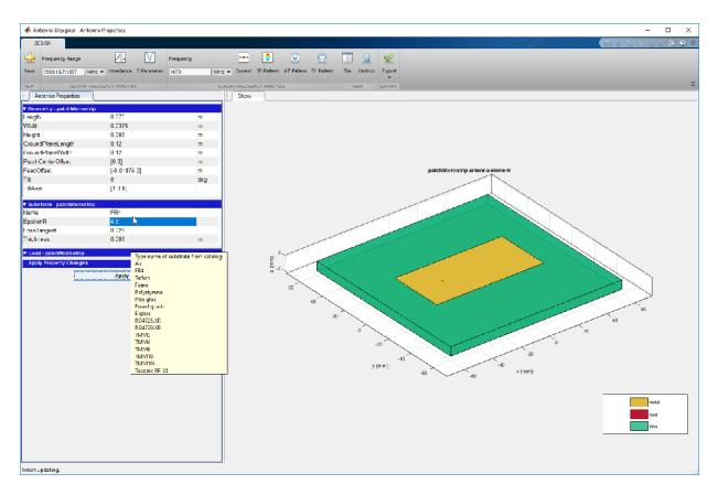
Click  ${\bf 3D}$  **Pattern** to plot the radiation pattern of the antenna at the default frequency of 1.67 GHz.
