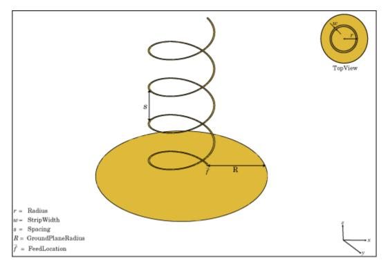
**Note** In an array of helix antennas, the circular ground plane of the helix is converted to rectangular ground plane.
