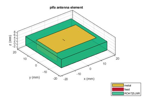
Calculate the impedance of the antenna over the specified frequency range. GHz. impedance(pf,linspace(2.2e9,2.5e9,31));
