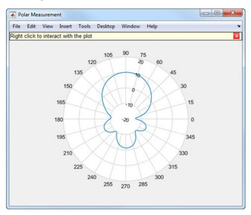
polarpattern class plots antenna or array radiation patterns in interactive polar format. You can also plot other types of polar data. Use these plots when interactive data visualization or measurement is required. Right-click the **Polar Measurement** window to change the properties, zoom in, or add more data to the plot.
