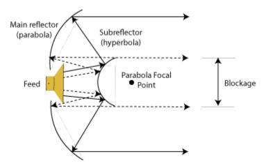
Focus of the main reflector and the near focus of the subreflector coincides. The energy is transmitted from the subreflector to the primary parabolic reflector. The parabolic reflector converts a spherical wavefront into a plane wavefront as the energy directed towards it appears to be coming from focus.
