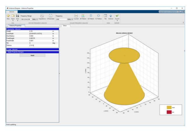
Calculate the S-parameter of the antenna at the specified frequency range.
