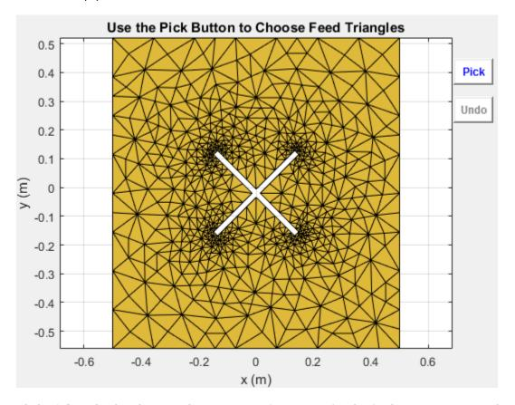
Click  $\mathbf{Pick}$  to display the cross-hairs. To specify a region for the feed point, zoom in and select two points, one inside each triangle on either side of the air gap. Select the points using the cross-hairs.
