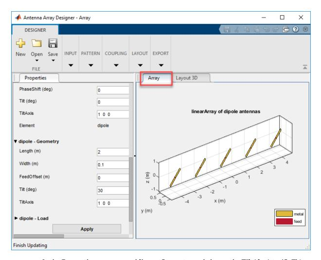
In the **Properties** pane, expand **linear-Geometry** and change the **Tilt(deg)** to 45. This changes the tilt of the entire array to 45 degrees.
