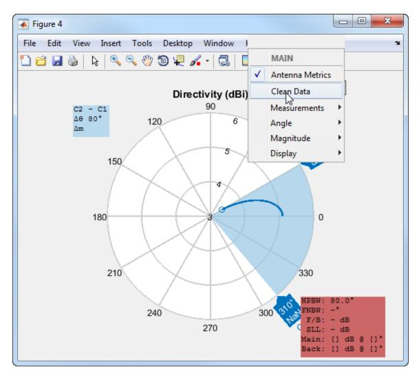
After using Clean Data, you see that the polarpattern beamwidth calculation matches the beamwidth plot calculation.
