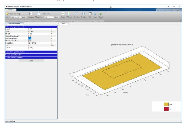
Add an FR4 dielectric as a substrate to the patch microstrip antenna. To add the dielectric, open the **Substrate** section and hover over the **Name** tab to see the **Dielectric Catalog**. Set the substrate **Name** to FR4, **EpsilonR** to 4.8000, and **Loss Tangent** to 0.0260. Click **Apply** to see the antenna.
