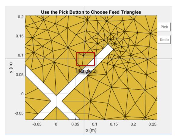
Selecting the second triangle creates and displays the antenna feed.
