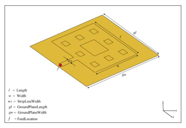
A fractal antenna uses a self-similar design to maximize the length or increase the perimeter of a material that transmits or receives electromagnetic radiation within a given volume or area. The main advantage of fractal antennas is that they are compact,
