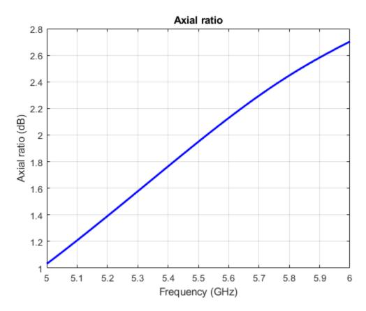
You can see from the axial ratio plot that the antenna supports circular polarization over the entire frequency range.
