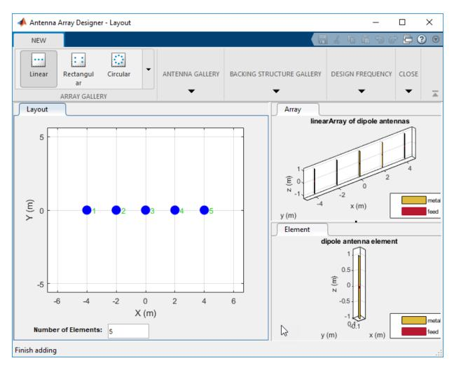
In the **Properties** pane, expand **dipole-Geometry** and change the **Tilt(deg)** to 30. This changes the tilt of each dipole element in the array to 30 degrees. Click on **Array** tab to view the array.
