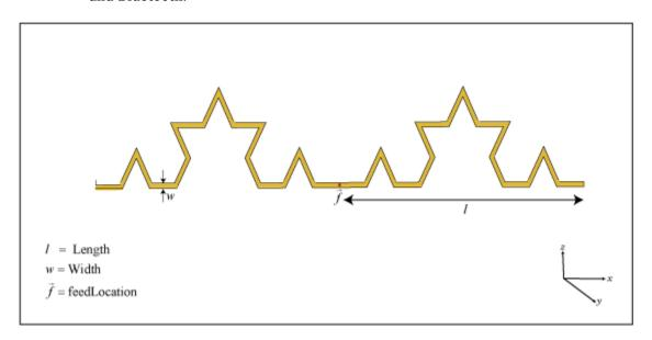
A fractal antenna uses a self-similar design to maximize the length or increase the perimeter of a material that transmits or receives electromagnetic radiation within a given volume or area. The main advantage of fractal antennas is that they are compact, which is an important requirement for small and complex circuits. Fractal antennas also have more input impedance or resistance due to increased length or perimeter, respectively.
