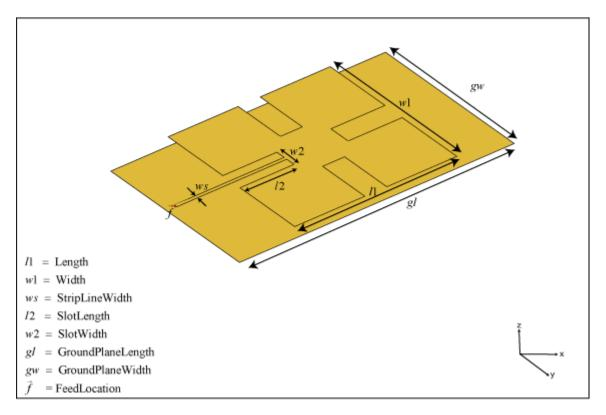
A fractal antenna uses a self-similar design to maximize the length or increase the perimeter of a material that transmits or receives electromagnetic radiation within a given volume or area. The main advantage of fractal antennas is that they are compact,
