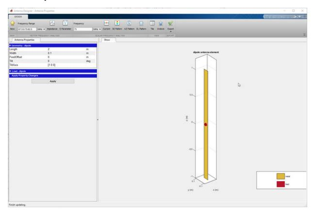
You can plot the **Impedance** and **S Parameter** of the antenna based on the specified **Frequency Range** in Hz.
