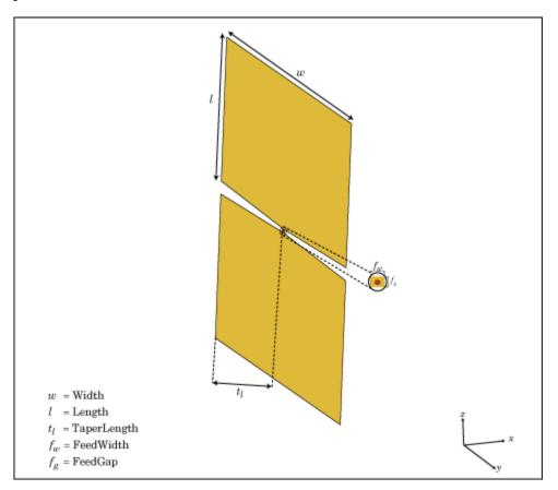
The width of the dipole is related to the circular cross-section by the equation,
