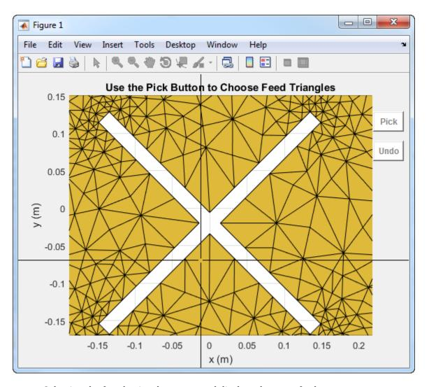
Selecting the fourth triangle creates and displays the array feeds.
