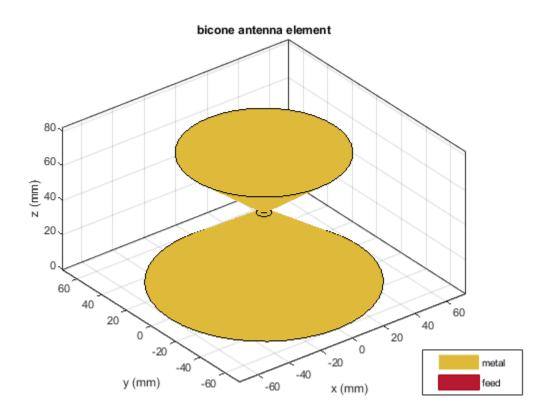
Calculate the impedance of the antenna over the frequency span of 500 MHz - 5 GHz. impedance(ant,linspace(0.5e9,5e9,51));
