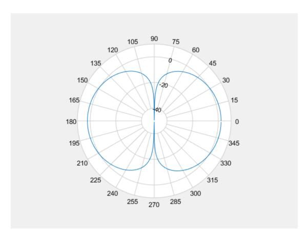
Create a cavity antenna. Calculate the directivity of the antenna at 1 GHz. Write the directivity of the antenna to cavity.pln using the msiwrite function.
