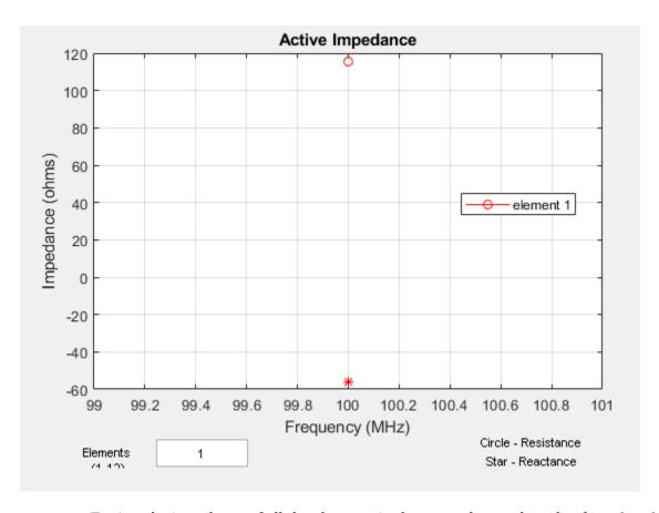
To view the impedance of all the elements in the array change the value from  ${\bf 1}$  to  ${\bf 1:12}$  as shown in the figure.
