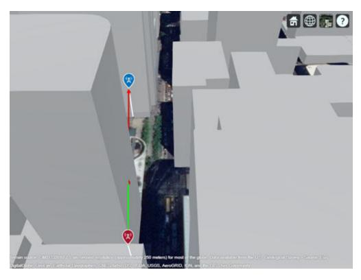
Show a reflected propagation path using ray tracing.
