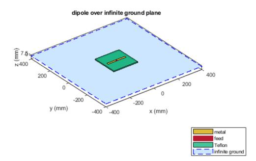
Calculate the radiation pattern of the antenna at 70 MHz. pattern(rf,70e6)
